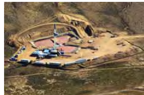
FIGURE I-27. CONVENTIONAL DRILLING SITE This site, with reserve pits disturbs 3-4 acres of land. Photo by Jonathan Selkowitz
